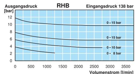
\*1 P<sub>1</sub> = 138 bar, P<sub>2</sub> = 10 bar und Δp = 3 bar
